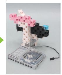
② Plug your servomotor cable into D9 and your battery box cable into the POWER port on the circuit board.
