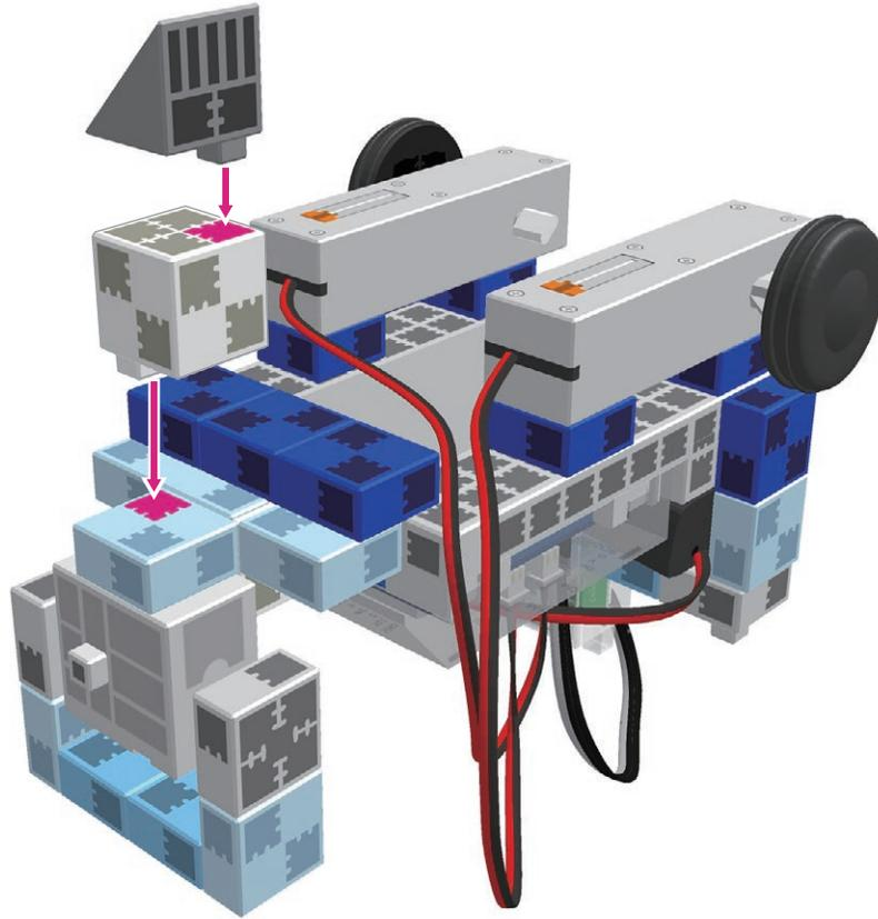
5 Connect the cables from servomotor **D11** to their corresponding place on your Studuino unit.
