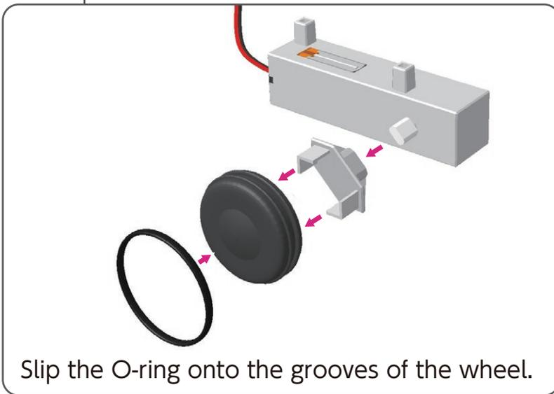
Slip the O-ring onto the grooves of the wheel.
