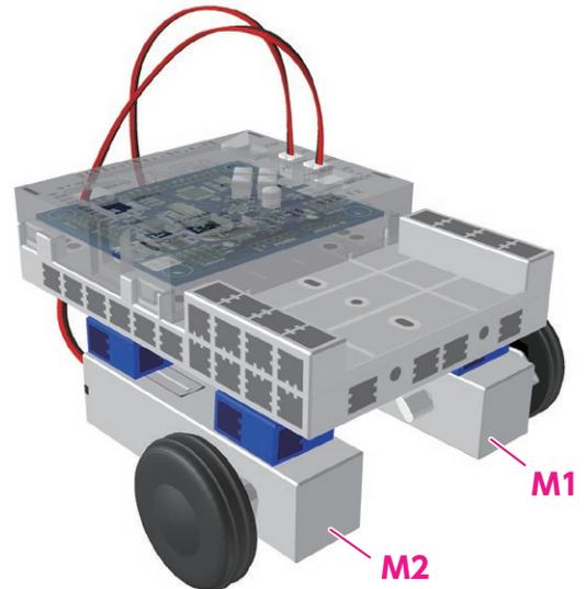
① Connect the assembled DC Motor to **M1**.
